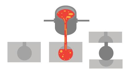
Casting also results in minimal material wastage, as it is not a subtractive manufacturing method where excess material is machined away, but rather only the specific amount of material required is poured in each time.
