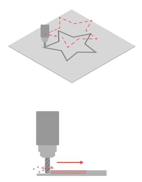
There are also various different kinds of mills, ranging from a 3-axis mill which can cut out simple shapes in the X, Y, and Z axes, all the way to 6-axis mills that can also rotate about those axes to create more complex curvatures.
