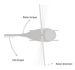
Sequence: Rotor/Tail, Show how the tail rotor works, then show how the control works for the main rotor
