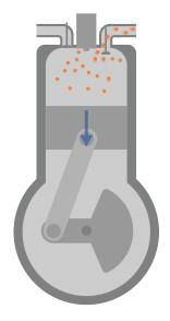
• When the piston reaches the top of this stroke, the exhaust valve is closed.
