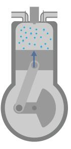
• As the piston reaches the top of its stroke, the spark plug creates a spark. The fuel and oxygen burn quickly. The cool liquid fuel becomes hot carbon dioxide and water vapor.
