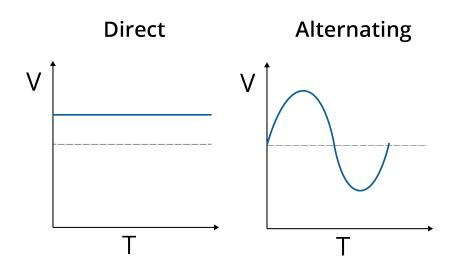
In most countries, the RMS of the voltage between 110 and 240 V. (The peak voltage is always  $\sqrt{2}$  times the RMS value. In the US, for example, people say "Our outlets supply 120 V." They mean that the RMS of the voltage difference between the wire and the earth is 120V. The peak voltage is almost 170V.)
