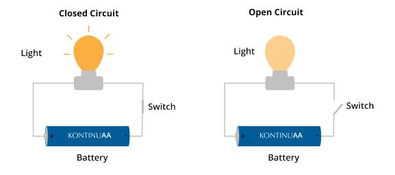
The lightbulb creates *Resistance* that the current pushes through. Think of it like plumbing: The current is the amount of water passing through a pipe. The resistance is something that tries to stop the current – like a ball of hair. The battery is what allows the current to push through the resistance; we call that pressure *voltage*.
