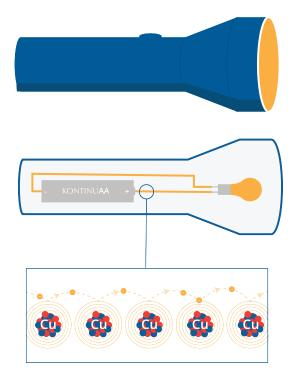
In some materials, like copper and iron, electrons are loosely bound to their nuclei, forming a sea of electrons, which allows energy to flow. These are good *electrical conductors*. In other materials, like glass and plastic, electrons don't leave their nuclei easily. Thus, they are terrible electrical conductors – we call them *electrical insulators*. For example, the plastic around a wire is electrical insulation.
