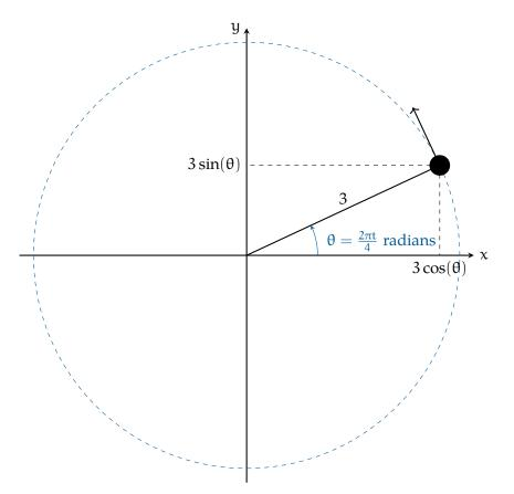
In this case, the radius, r, is 3 meters. The period, T is 4 seconds. In general, we say that circular motion is given by:
